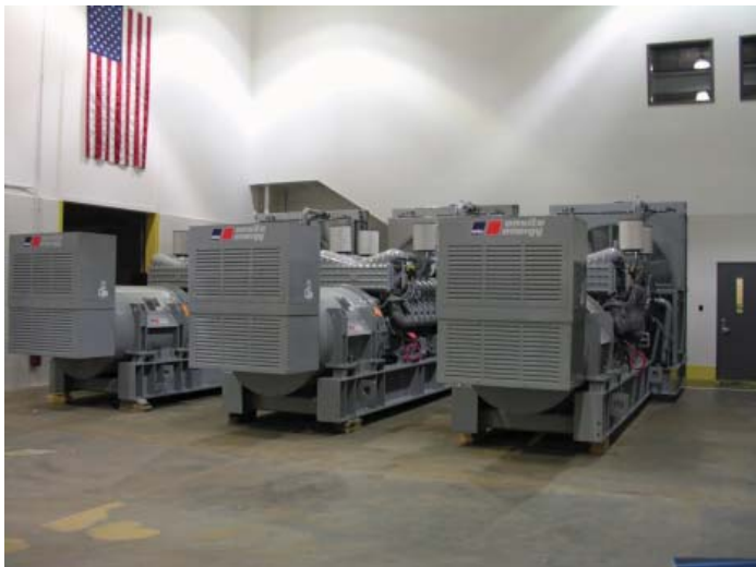
Three of six units, awaiting shipping to the new WORLD TRADE CENTER..2500 Kva
